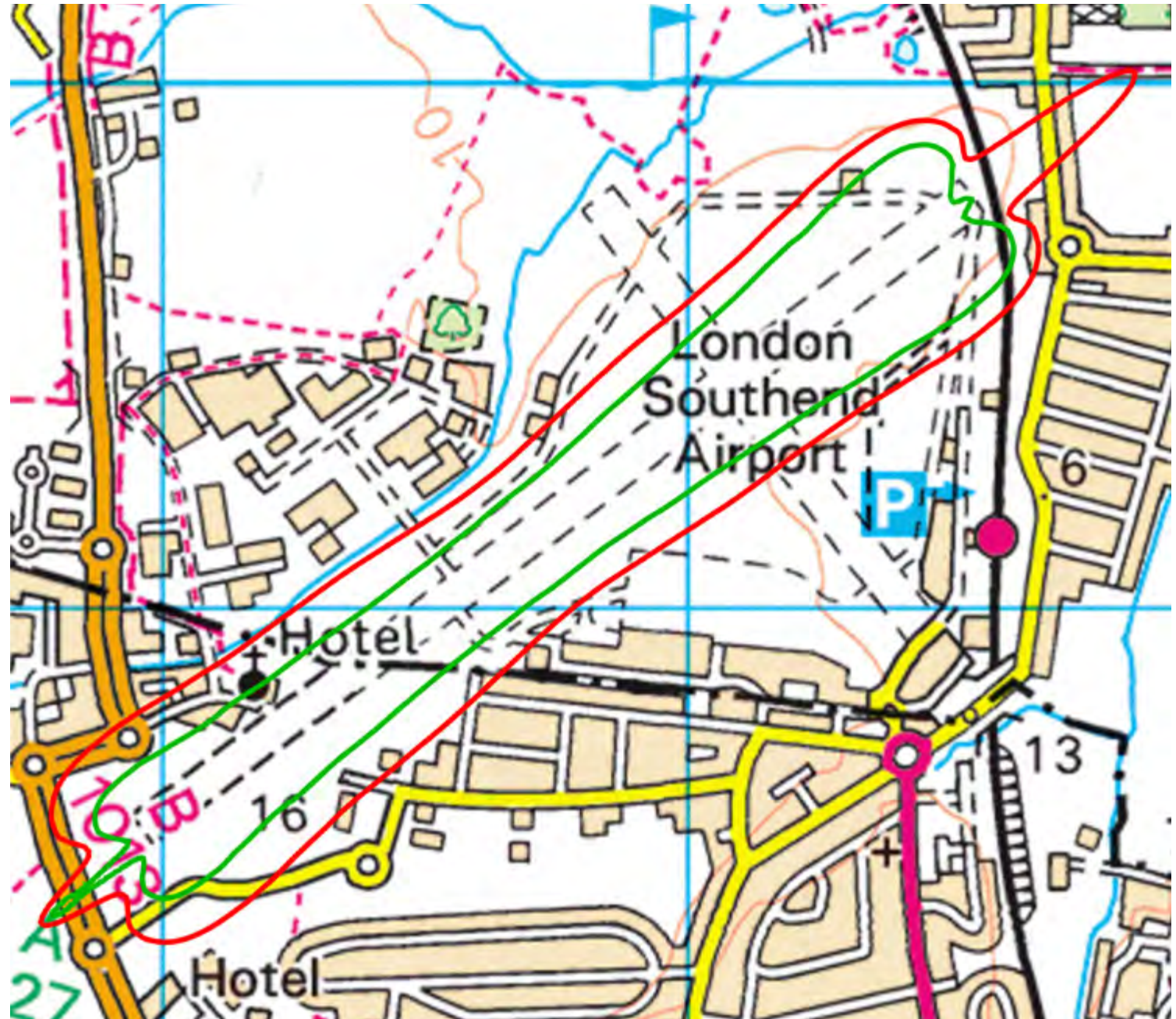
Figure A London Southend Airport summer noise contours 2020. Airborne aircraft noise contours summer average daytime. Contour comparison 2018/2020 – 63dB. This drawing contains Ordnance Survey data © Crown Copyright and database right 2014.
